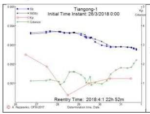
This figure presents the ballistic coefficient estimates, the values of the geomagnetic disturbance index (*Kp*) and the minimized criterion for all preceding time instants of orbital parameters updating in interval from March 26 to March 31. The estimates of ballistic coefficient (Sb) have changed within the range from 0.00369 to 0.00276 m²/kg, i.e. 1.34 times. The highest drag variations have been observed after March 28, which is the consequence of reduction of geomagnetic activity
