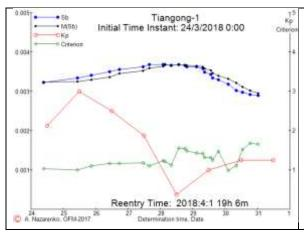
This figure presents the ballistic coefficient estimates, the values of the geomagnetic disturbance index (*Kp*) and the minimized criterion for all preceding time instants of orbital parameters updating in interval from March 24 to March 30. The estimates of ballistic coefficient (Sb) have changed within the range from 0.00369 to 0.00290 m²/kg, i.e. 1.27 times. The highest drag variations have been observed after March 28, which is the consequence of reduction of geomagnetic activity
